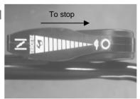
Figure 8. Throttle Control - ("CHOKE" | | Position)
